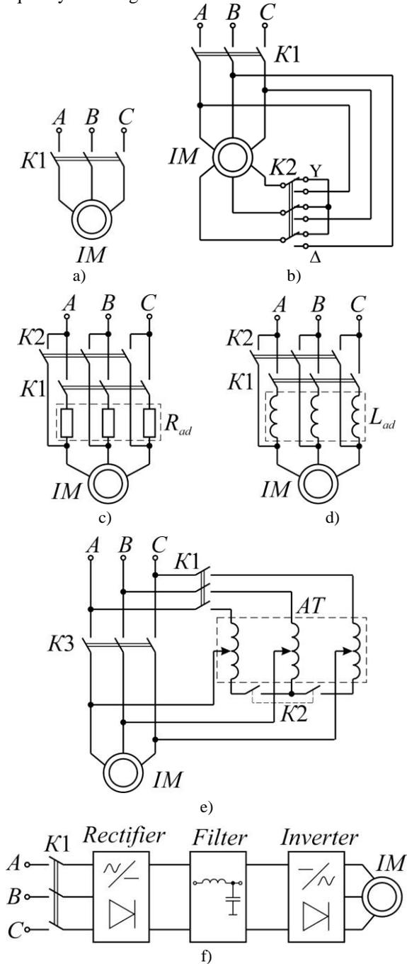
Figure 1. Electric circuits of IM starting:
