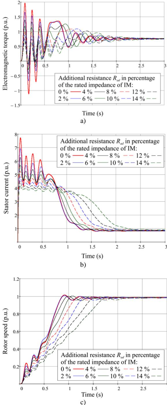
Figure 4. Additional resistance starting transient curves.
