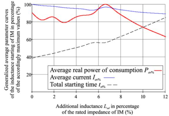
Figure 7. Generalized characteristics of an additional inductance starting.
