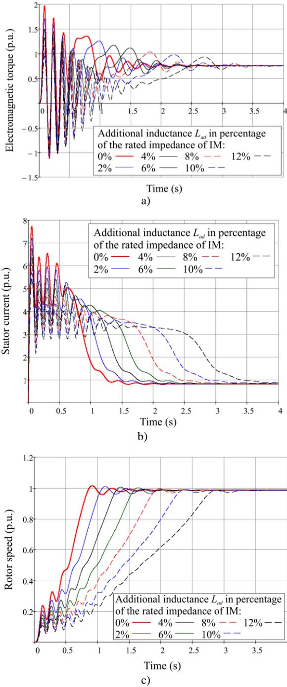
Figure 6. Transient curves of an additional inductance IM starting.
