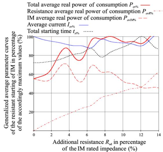
Figure 5. Generalized characteristics of the additional IM starting resistance.
