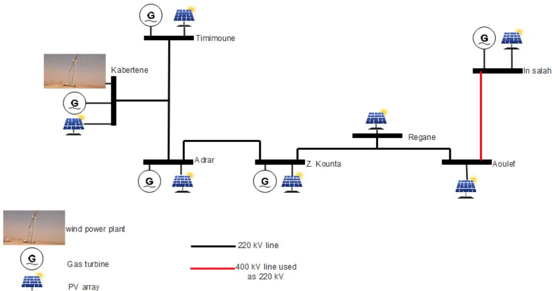
Figure 3. The PIAT single line diagram
