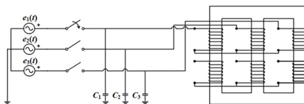
Figure 1. Ferroresonance of a three-phase three-legged power transformer – switching-on phase 1.
