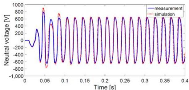
Figure 9. Neutral point voltage: simulation vs. measurement (Variant 1).
