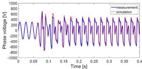
Figure 11. Phase 1 voltage: simulation vs. measurement (Variant 2).
