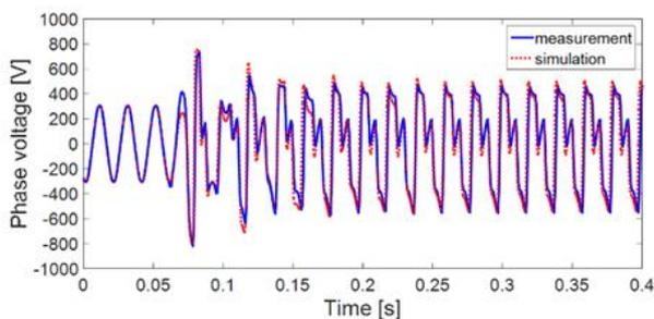
Figure 12. Phase 2 voltage: simulation vs. measurement (Variant 2).
