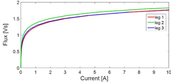
Figure 4. Nonlinear magnetizing curves of the three transformer legs.
