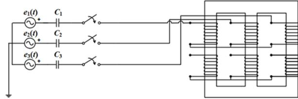
Figure 2. Ferroresonance of a three-phase three-legged power transformer – simultaneous switching-on the phases.
