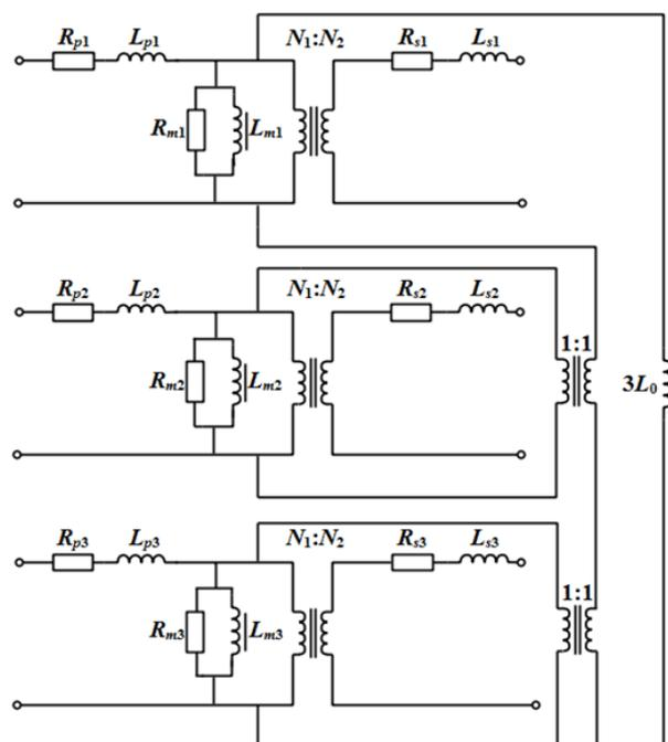
Figure 3. Equivalent circuit of a three-phase three-legged transformer.
