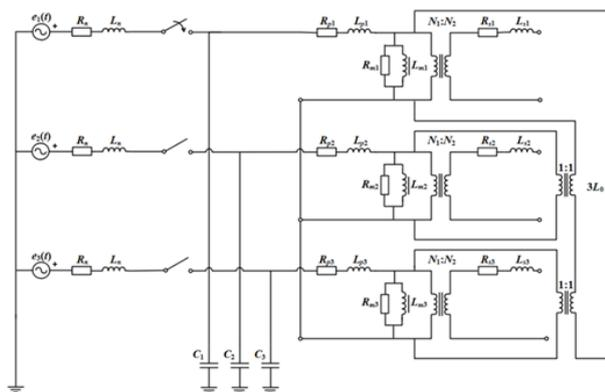
Figure 5. Equivalent circuit of the ferroresonant system – Variant 1.
