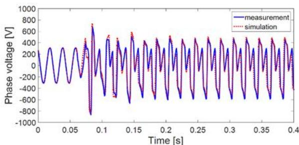
Figure 13. Phase 3 voltage: simulation vs. measurement (Variant 2).
