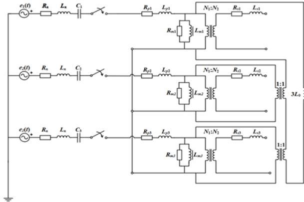
Figure 10. Equivalent circuit of the ferroresonant system – Variant 2.
