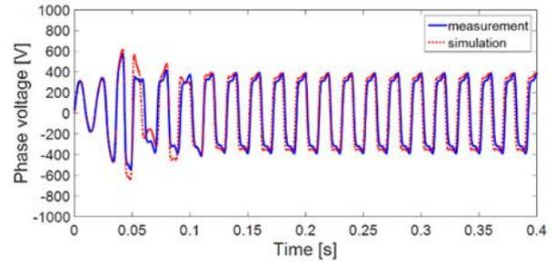
Figure 6. Phase 1 voltage: simulation vs. measurement (Variant 1).
