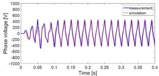
Figure 7. Phase 2 voltage: simulation vs. measurement (Variant 1).
