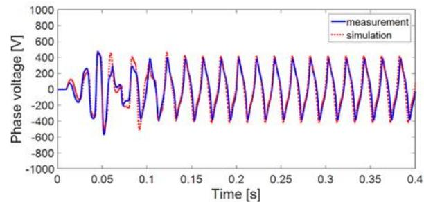
Figure 8. Phase 3 voltage: simulation vs. measurement (Variant 1).
