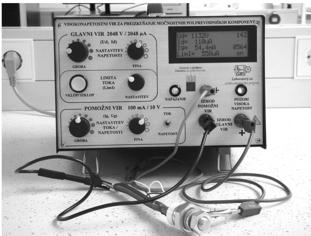
Figure 12. Laboratory prototype of the developed high-voltage DC source with SCR under test
