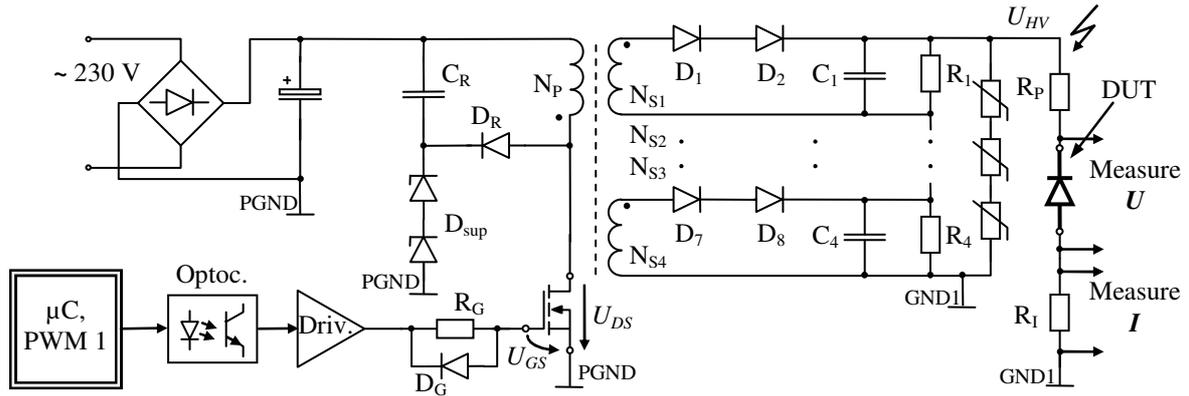
Figure 3. Topology of the flyback switching converter with the high-voltage output
