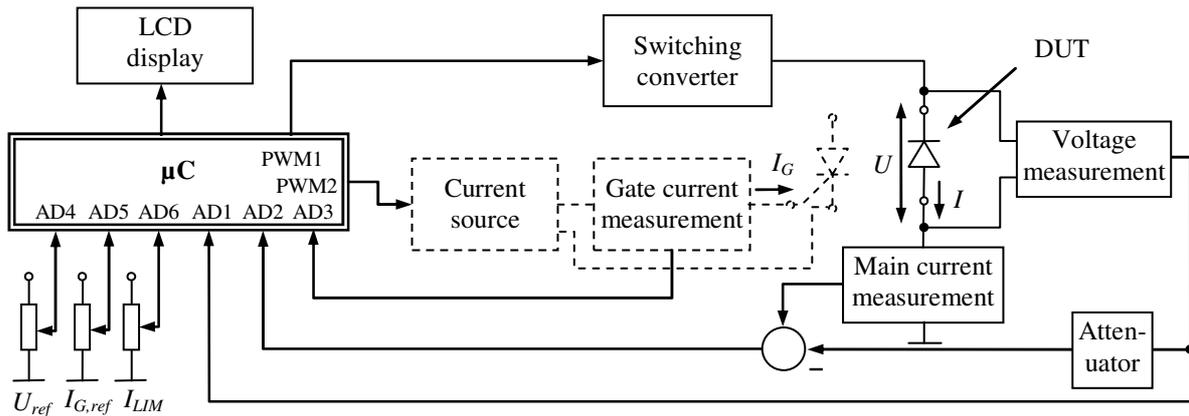
Figure 1. Block diagram of the proposed high-voltage DC source
