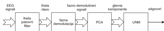
Slika 4.: Bločni diagram obdelave signalov pri nalogah delovnega spomina Figure 4.: Block diagram of working-memory task signal processing
