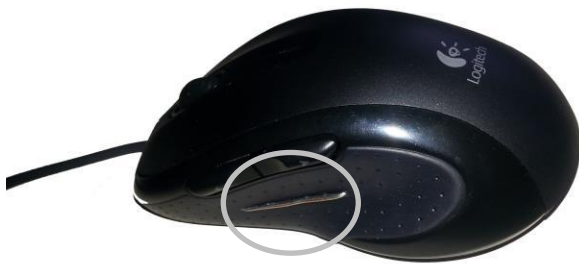
Figure 10. Measurements of the student's well-being while solving a computer-based school test in distance learning. A student uses a computer mouse, equipped with electrodes (encircled) to non-intrusively measure the student's EDA.
