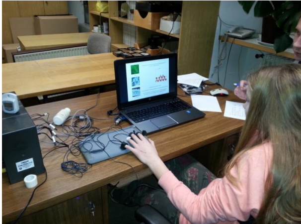
Figure 1. Measurement of the impact of performing demanding science tests on the student's physiology - heart rate, skin conductance and finger temperature on a non-dominant arm, and respiratory [16].
