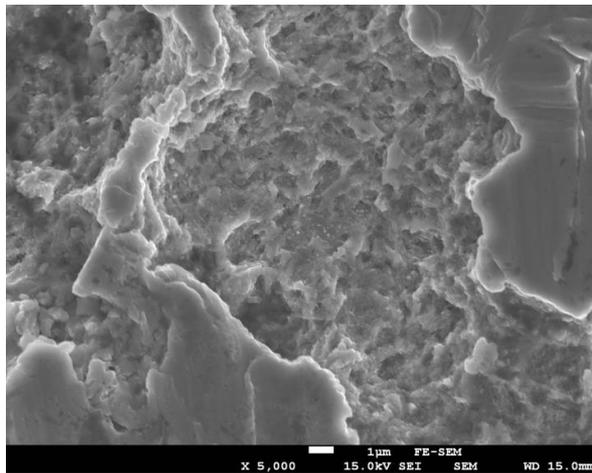
Figure 2. SEM electron image of the intergranular fracture of robot laser hardened specimen.
