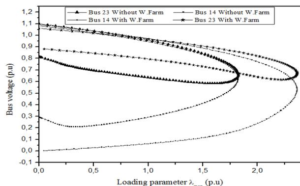
Figure 17. P-V curves for bus 14 and 23 for the base case and after a wind farm inclusion.
