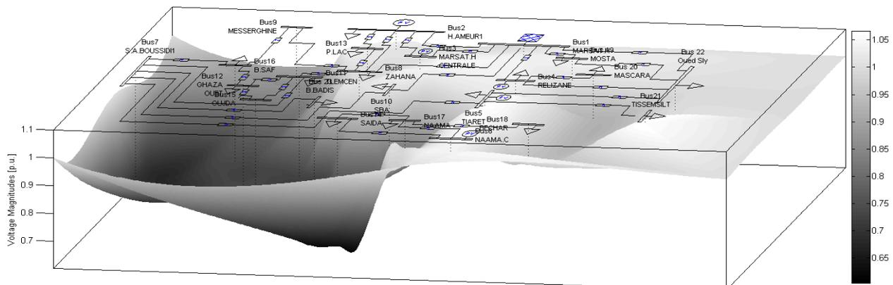
Figure 7. Three-dimensional voltage profiles before adding the wind farm.
