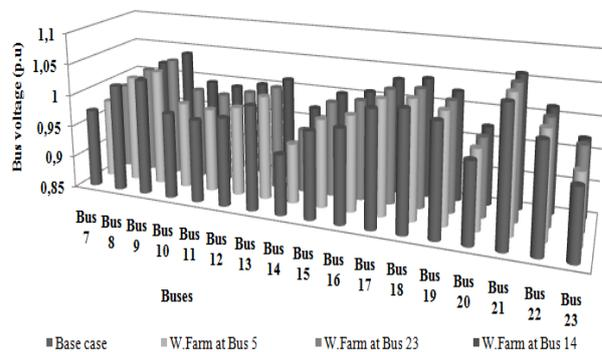
Figure 13. Bus voltages in the base case and with the integration of a wind farm.
