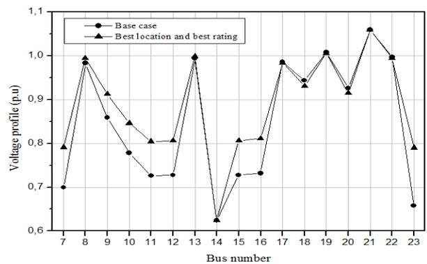
Figure 16. Bus voltages at a critical state before and after a wind farm inclusion.
