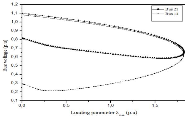
Figure 10. PV curve for critical nodes.
