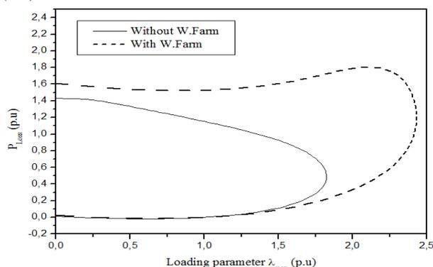
Figure 18. Variation in the active-power losses as a function of the loading parameter ( $\lambda$ ).
