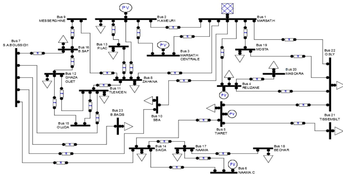
Figure 5. Western Algerian 220 KV electric power system (2016).
