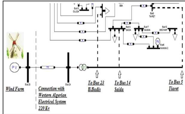
Figure 11. Connection of the wind farm with the electric power system.
