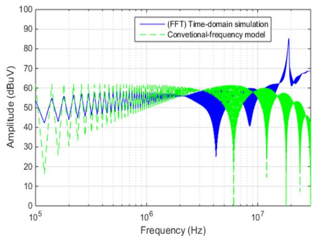
Figure 5. Conventional CM EMI noise spectrum.
