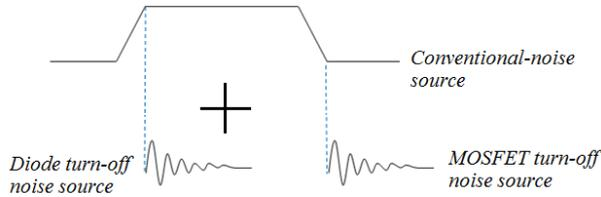
Figure 6. Decomposition of the waveform noise source in a DC/DC buck converter.
