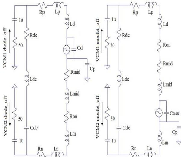
Figure 9. CM high-frequency equivalent circuits during a switching transient (a) diode turn-off (b) MOSFET turn-off [5].
