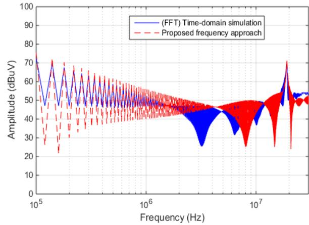
Figure 10. DM EMI noise-voltage spectrum.
