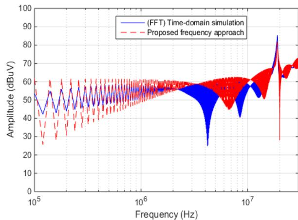
Figure 11. CM EMI noise-voltage spectrum.
