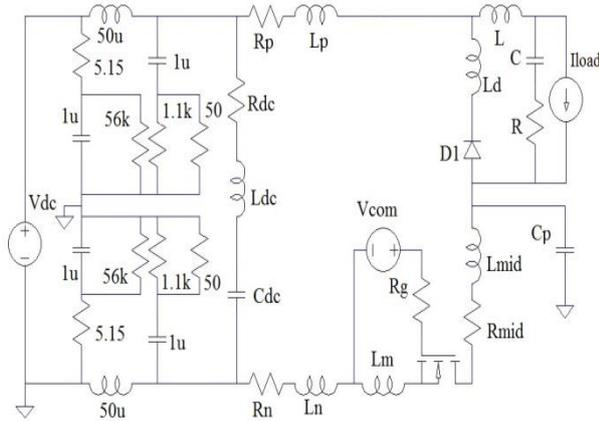
Figure 1. Time-domain simulation circuit of a buck converter connected to LISN [4, 5].
