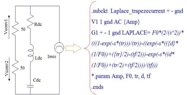
Figure 2. Conventional DM EMI Model [4, 5, 10].
