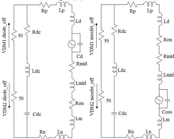
Figure 7. DM high-frequency equivalent circuits during a switching transient (a) diode turn-off (b) MOSFET turn-off [5].
