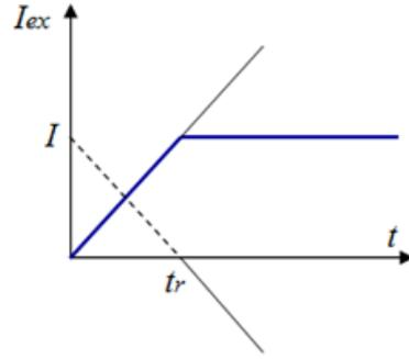
Figure 8. Excitation source during a switching transient [5, 12].
