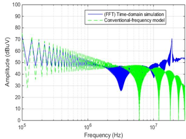
Figure 4. Conventional DM EMI noise spectrum.
