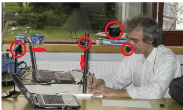
Figure 4: Simultaneous capture of three live pictures: writing, auditorium, talking face, and capture of selected voice for transmission in a tele-lecturing session
