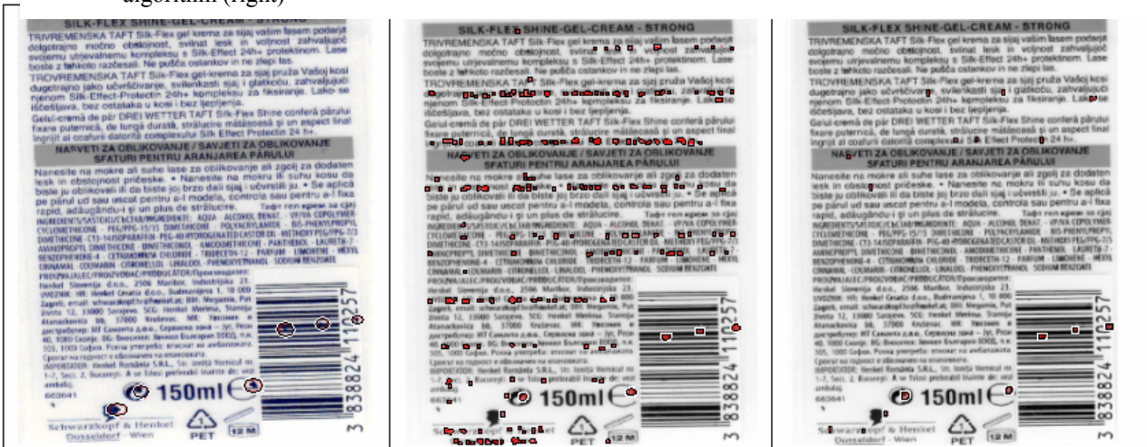
Slika 5: Primer analize za motiv »Silk-flex«: napake, najdene s prostim očesom (levo), in posamezne napake, najdene s pomočjo programa (sredina) ter združene v regije (desno) Figure 5: Printing error detection for document "Silk-flex": errors as seen by a human observer (left), found by our algorithm (middle), and grouped into erroneous regions (right)
