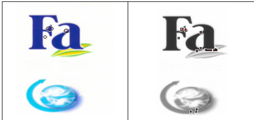
Slika 4: Primer analize za motiv »Fa«: napake, najdene s prostim očesom (levo), in napake, najdene s pomočjo programa (desno) Figure 4: Printing error detection for label "Fa": errors as seen by a human observer (left), and found by our algorithm (right)
