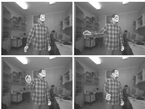
Figure 3. Example of final segmentation results. The detected region contours are marked in white.
