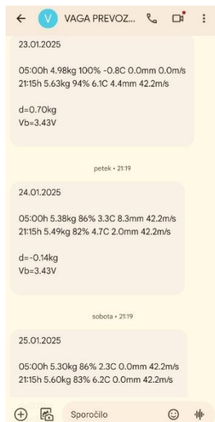
Figure 4. Data received from an IoT scale displayed on a mobile phone interface.
