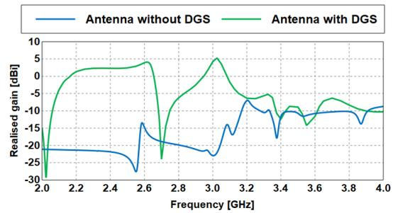
Figure 7. Gain of the antenna with and without IPM-DGS at  $\theta = 0^\circ$ .
