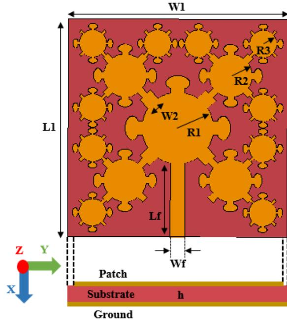
Figure 1. Structure of the corona-fractal antenna design.
