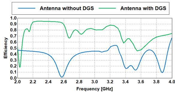
Figure 10. Radiation efficiency of the antennas (with and without IPM-DGS).
