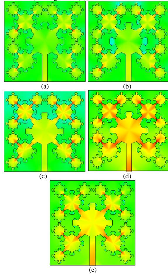
Figure 11. Surface current distribution of the antenna with IPM-DGS at (a) 2.62 GHz, (b) 3.02 GHz, (c) 3.35 GHz, (d) 3.5 GHz and (e) 3.62 GHz.
