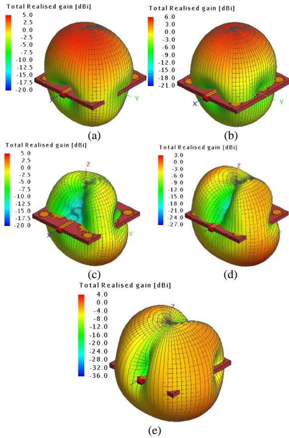
Figure 9. 3D total radiation pattern of the antenna with IPM-DGS at (a) 2.62 GHz, (b) 3.02 GHz, (c) 3.35 GHz, (d) 3.5 GHz and (e) 3.62 GHz.
