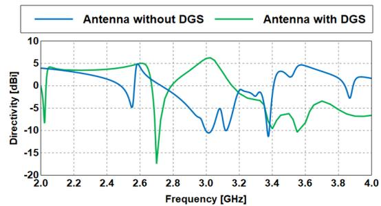
Figure 8. Antenna directivity with and without IPM-DGS at  $\theta = 0^\circ$ .
