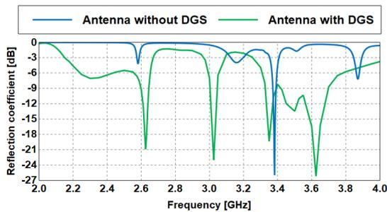
Figure 4. Reflection coefficients of the antenna with and without IPM-DGS.
