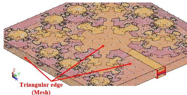
Figure 3. Simulation mesh produced by FEKO.
