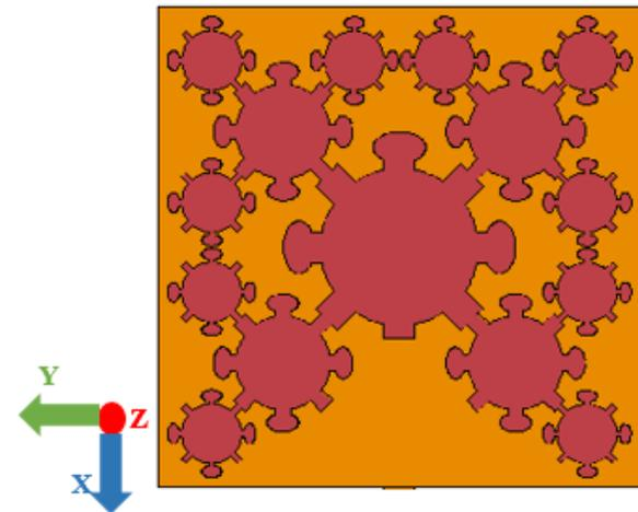
Figure 2. Ground with IPM-DGS.
