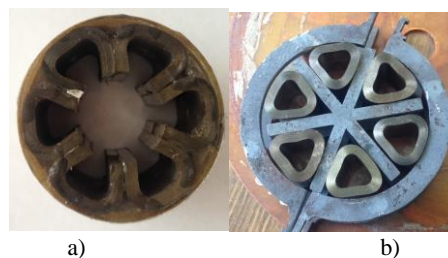
Figure 1. AMM core created by the proposed technology (a) and triangular cores in the technological mandrel (b)
