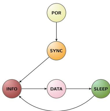
Figure 5. BLEER routing algorithm state machine.
