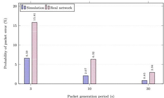
Figure 9. Node N1 packet loss as a function of the traffic generation parameter.
