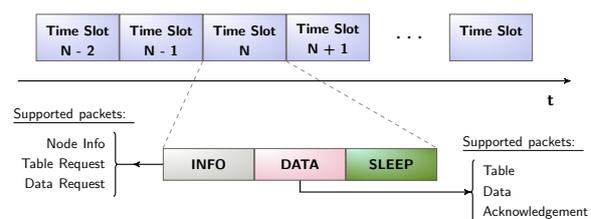
Figure 3. BLEER algorithm time slotted medium access. time slots are divided into three regions: INFO, DATA
