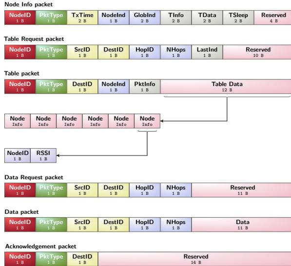
Figure 4. Packet structure of supported BLEER packets.
