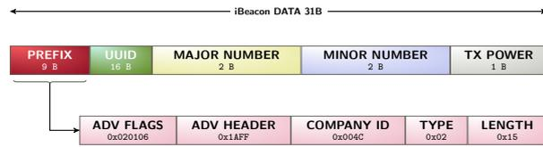
Figure 1. Apple iBeacon packet structure.
