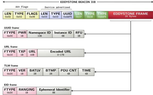
Figure 2. Eddystone beacon packet structure.
