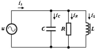
Figure 1. Simplified parallel ferroresonant circuit.
