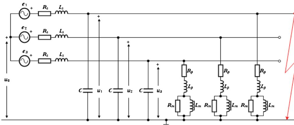
Figure 5. Equivalent model of ferroresonance in a three-phase isolated network: the case of initiation and elimination of single-phase short circuits.
