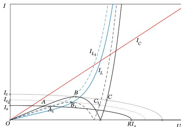
Figure 4. Nonlinear curves of a parallel ferroresonant circuit: the case of changing (decreasing) the inductance nonlinear curve.
