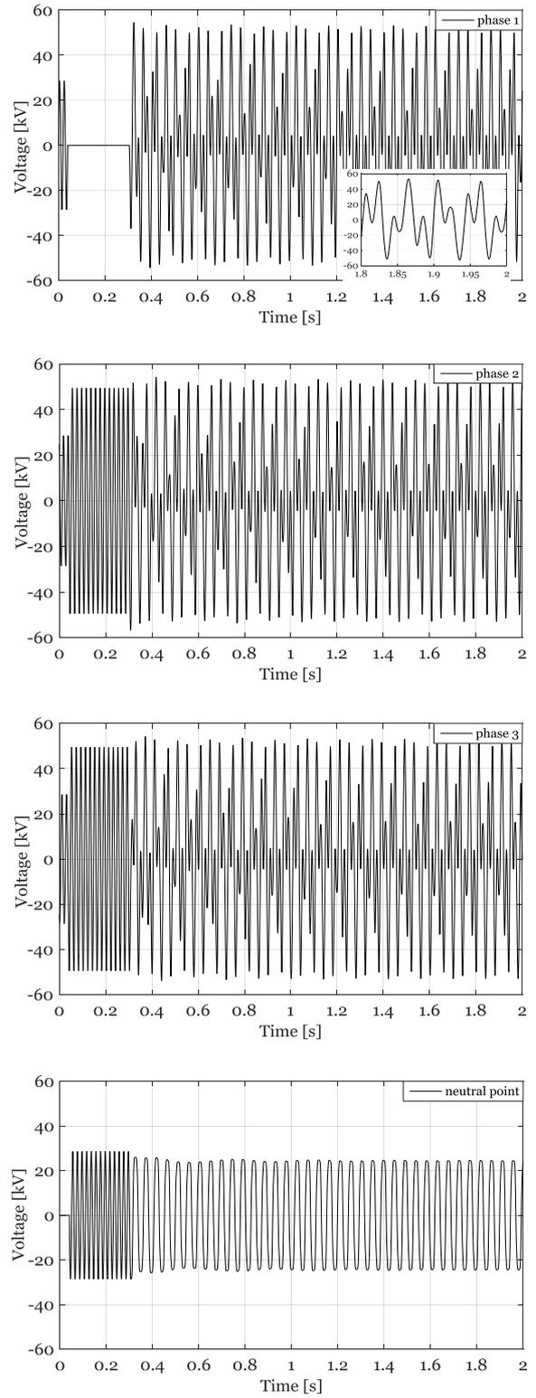
Figure 7. Phase voltages and voltage of the neutral point, two inductive voltage transformers,  $C = 150 \text{ nF}$ .
