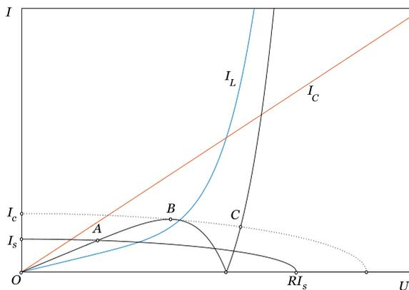
Figure 2. Nonlinear curves of a parallel ferroresonant circuit: basic case.
