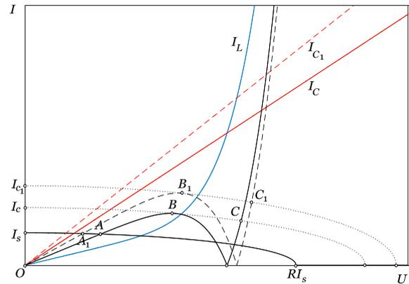
Figure 3. Nonlinear curves of a parallel ferroresonant circuit: a case of an increased system capacitance.
