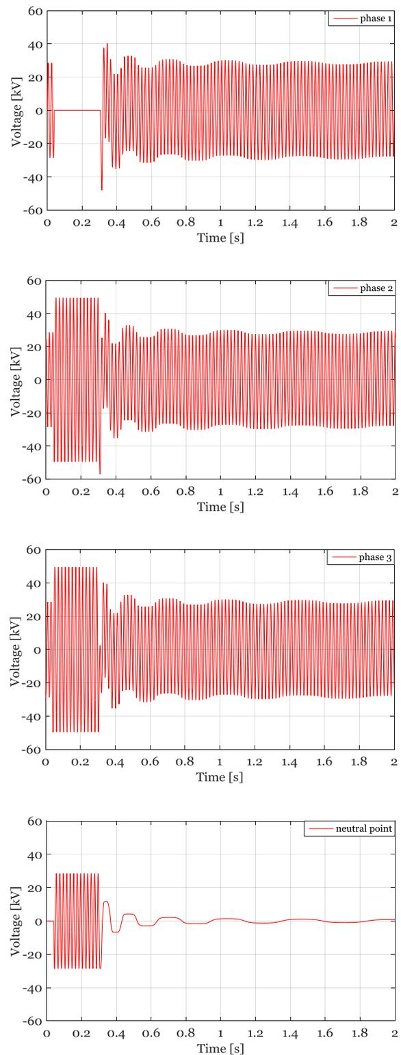
Figure 8. Phase voltages and voltage of the neutral point, two inductive voltage transformers,  $C = 575 \text{ nF}$ .
