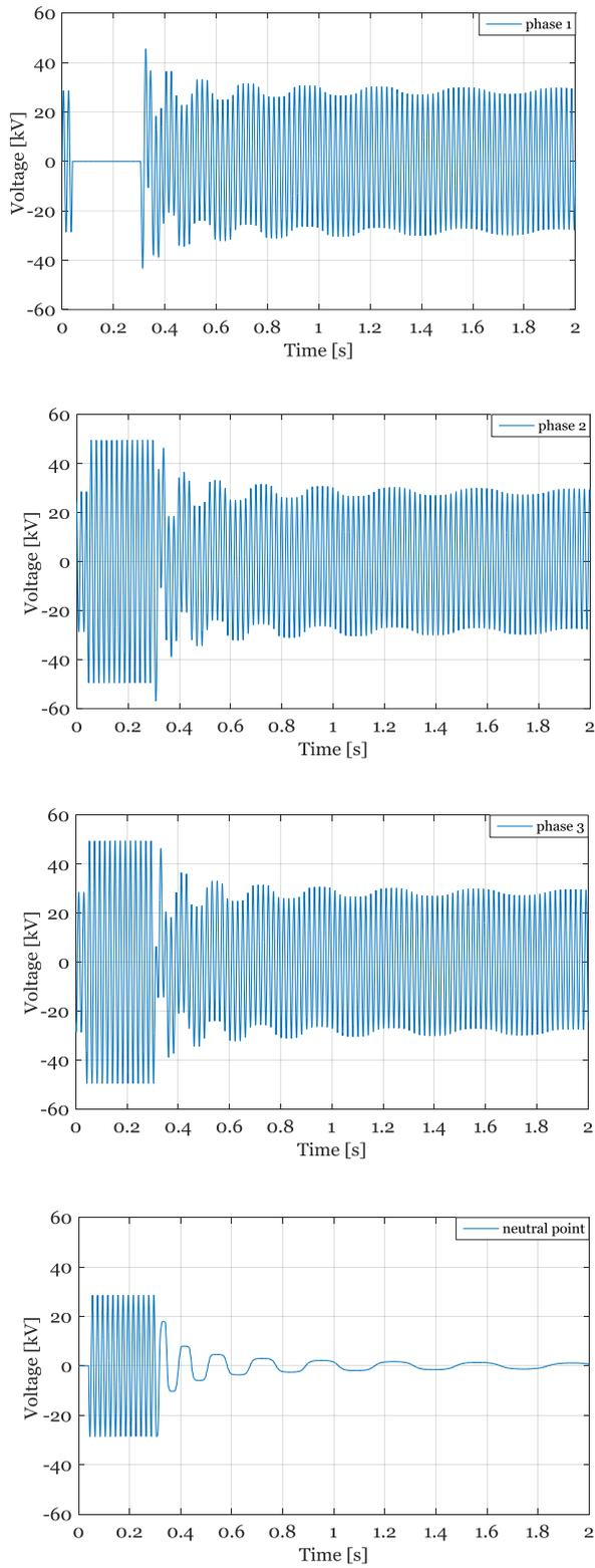
Figure 6. Phase voltages and the voltage of the neutral point, one inductive voltage transformer,  $C = 150 \text{ nF}$ .
