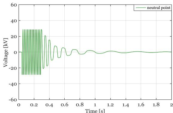
Figure 9. Neutral point voltage, two inductive voltage transformers,  $C = 150 \text{ nF}$ , the damping resistor connected.
