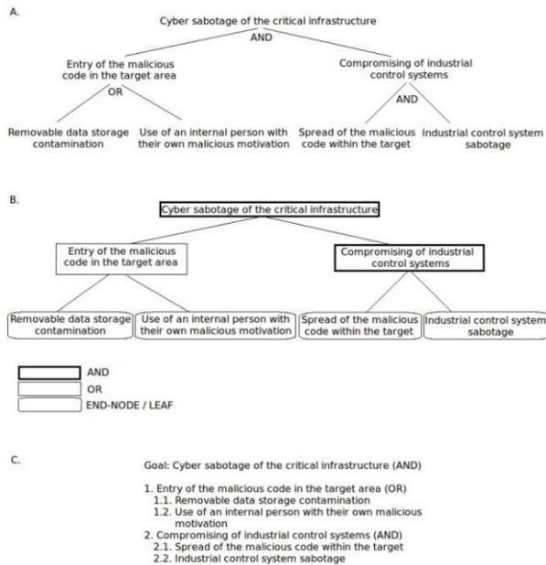
Figure 1. Same attack tree represented in two graphic variations (A. and B.), and the attack tree in a textual form (C.).
