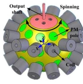
Figure 3: Spinning motion
