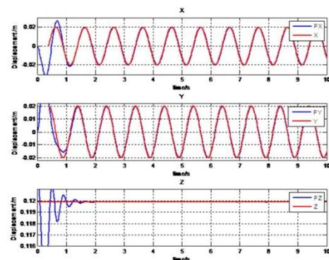
Figure 15. Angle-displacements tracking curve
