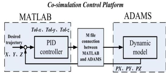
Figure 13. Structure of the co-simulation control platform
