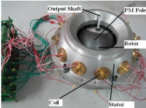
Figure 1. Basic mechanical structure of PMSA
