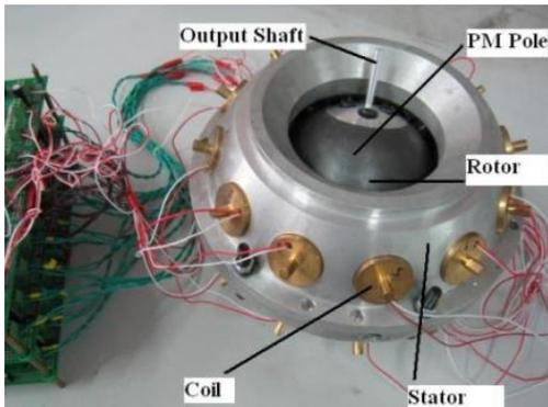
Figure 1. Basic mechanical structure of PMSA
