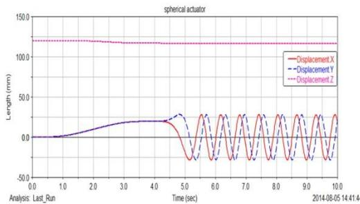
Figure 6. Output angle-displacements curve
