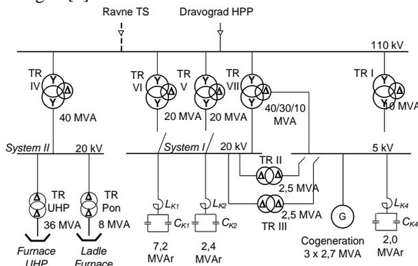
Figure 1: Simplified unipolar scheme of the Ravne power network.
