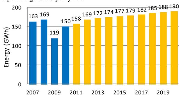
Figure 4: Total active-power consumption in the area of the Ravne network (current and foreseen).
