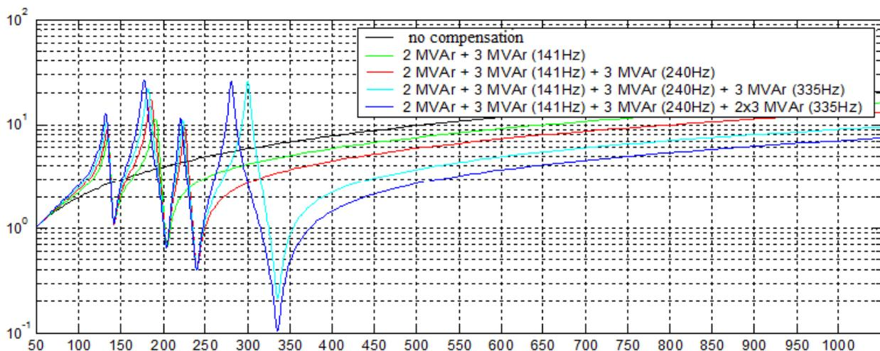
Figure 5: Frequency characteristic of the network impedance at the 20 kV busbar system.
