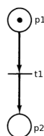
Figure 1: Example of a simple PN that describes translation. Place p_1 presents mRNA , place p_2 expressed protein and transition t_1 the reaction of translation.
