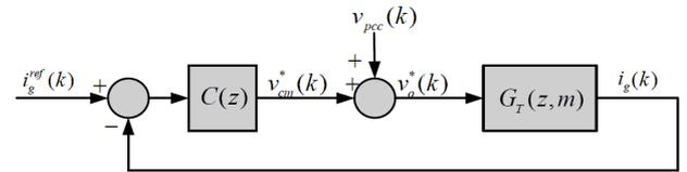
Figure 9. The closed-loop block diagram of the current tracking loop.
