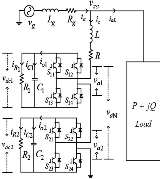
Figure 1. Block diagram of the cascaded H-bridge multilevel DSTATCOM.
