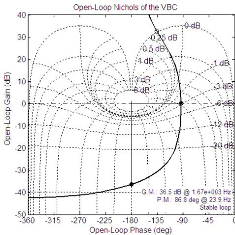
Figure 11. The open-loop Nichols diagram of the voltage balancing controller (VBC) when  $T_c=100\mu s$ .
