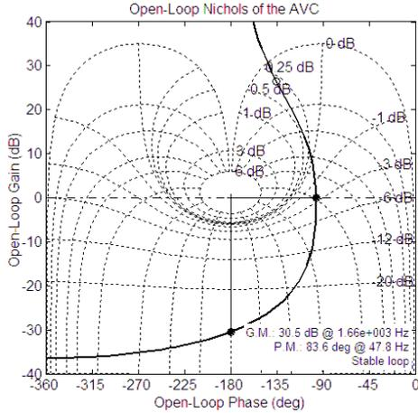
Figure 10. The open-loop Nichols diagram of the average voltage controller (AVC) when  $T_c=100\mu s$ .
