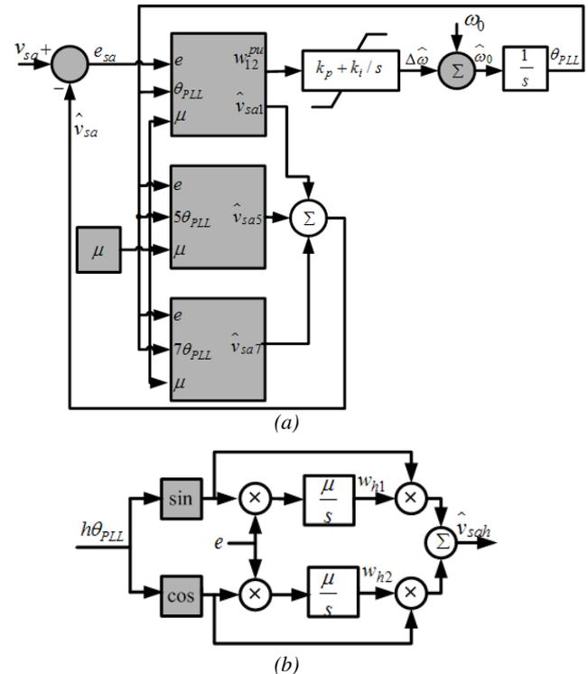
Figure 8. The proposed ADALINE-PLL (APLL) (a) overview of the APLL;(b)the block diagram for the  $h$ th order harmonic component
