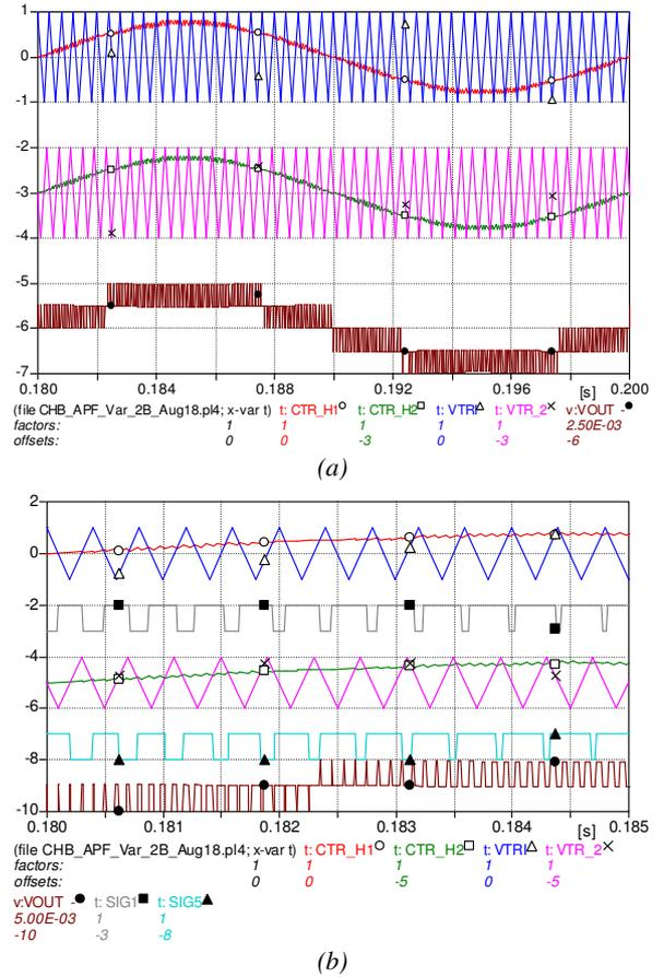
Figure 2. The simulated waveforms of the CHB-DSTATCOM: (a) The waveform of the modulation signal, phase-shifted carriers and the output multilevel voltage; (b) The enlarged view of (a) including the gating signals of the first IGBT for each H-bridge inverter.
