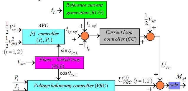
Figure 7. The block diagram of the devised control algorithms.
