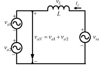
Figure 3. The equivalent circuit diagram of the CHB-DSTATCOM.
