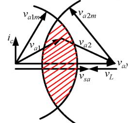
Figure 5. The stable control area of the CHB-DSTATCOM.
