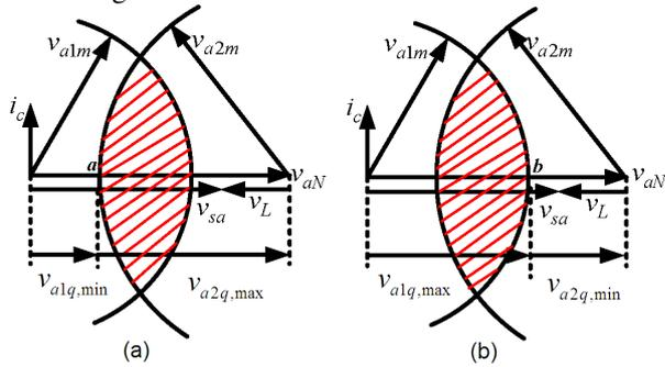
Figure 6. The diagram of maximum and minimum reactive power limits.
