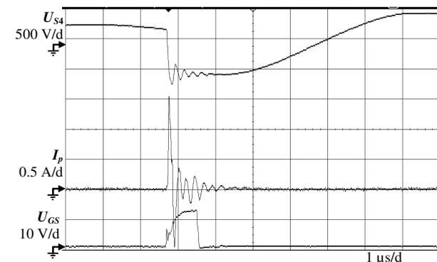
Figure 8. Waveforms of the unloaded source at a normal MOSFET turn-on speed,  $D = 3.3$  %
