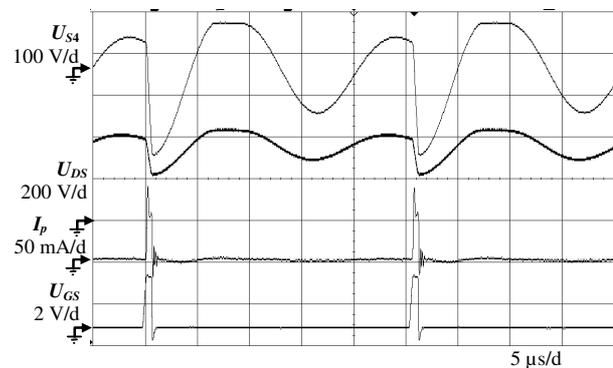
Figure 7. Waveforms of the unloaded source at a decreased MOSFET turn-on speed,  $D = 3.3$  %
