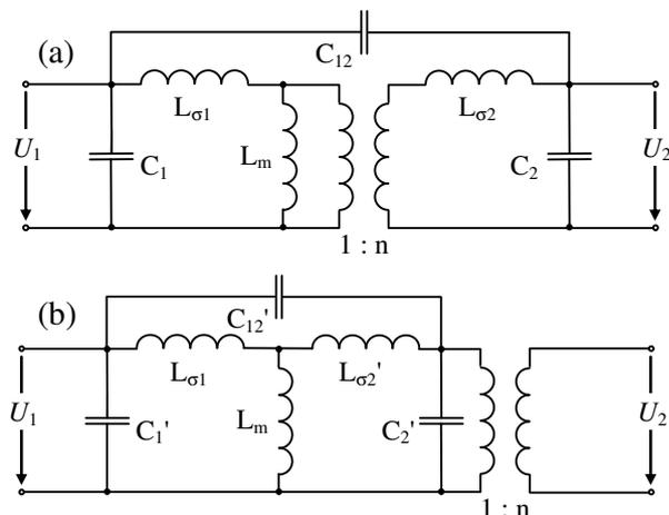
Figure 4. Equivalent circuit of a two-winding high-frequency transformer (a), as referred from the primary side (b)
