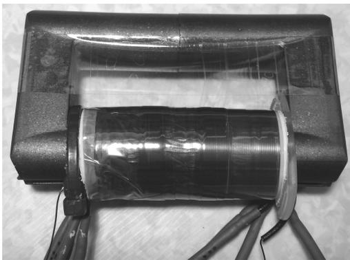
Figure 5. Photograph of used flyback transformer of primary current  $I_p$  charges the parasitic capacitor and the second part heaps the magnetic energy in the ferrite core of the flyback transformer.
