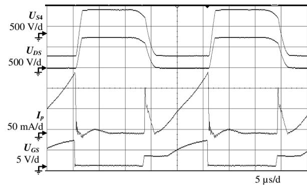
Figure 6. Waveforms of the loaded source,  $D = 50$  %
