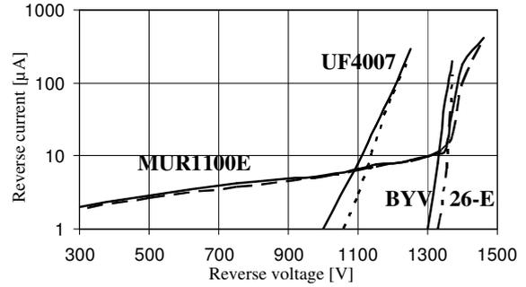
Figure 11. Reverse current versus the reverse voltage for similar ultra fast diodes
