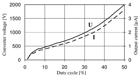
Figure 10. Source output current and the switching converter output voltage at short-circuited output terminals
