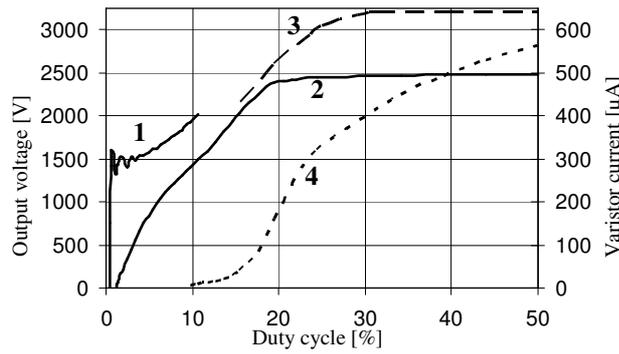
Figure 9. Graphs of the source output voltage: 1-normal MOSFET turn-on, 2/3-turn-on at a decreased speed with/without protecting varistors and 4-varistor current
