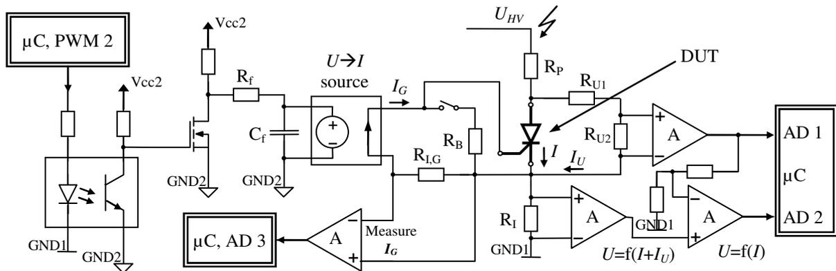
Figure 2. Topology of the measuring units used for the proposed high-voltage source
