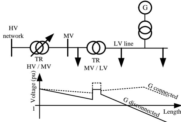
Figure 1: Voltage profile of a radial distribution line with DG units.
