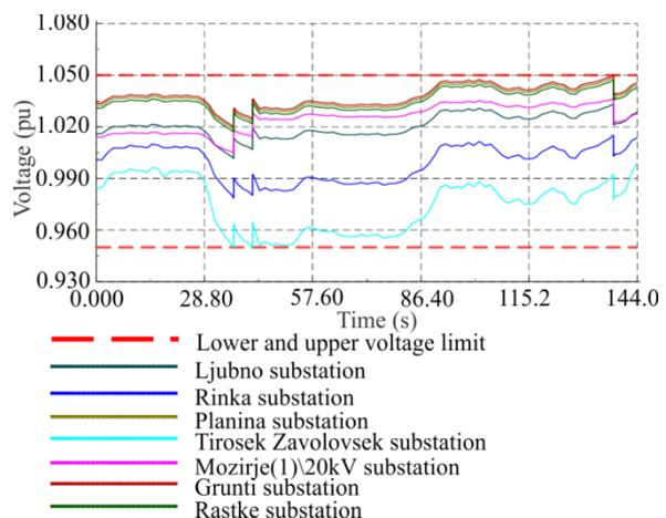
Figure 11: Central voltage control and reactive-power control – MP voltages.
