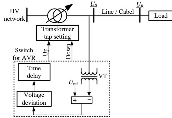
Figure 6: Classical voltage - control concept in RTP.
