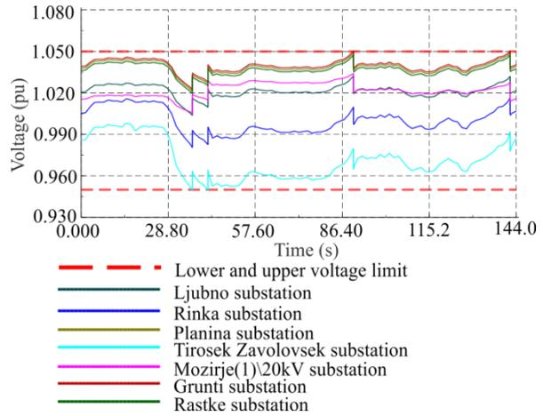
Figure 10: Central voltage control – MP voltages.
