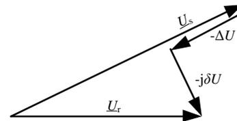
Figure 3: Voltage phase diagram.
