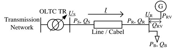
Figure 2: Simple network with a DG unit.
