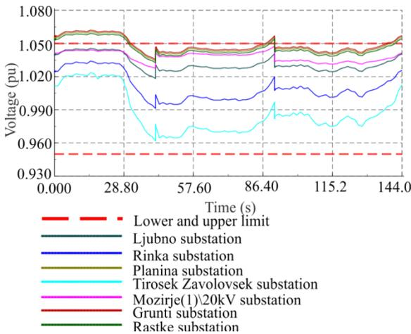
Figure 9: Classical voltage control and reactive-power control – MP voltages.
