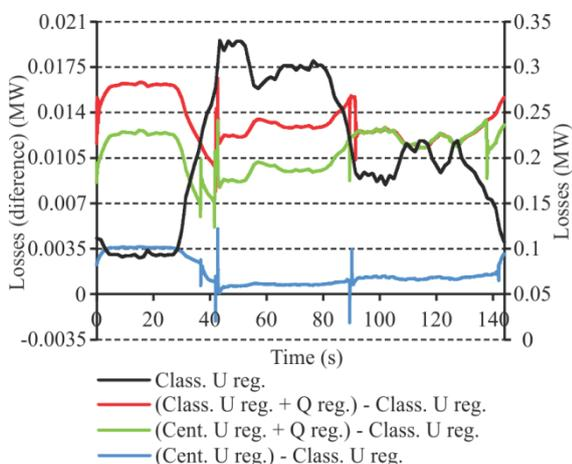
Figure 12: Losses in classical voltage control and differences between the classical and other control strategies.
