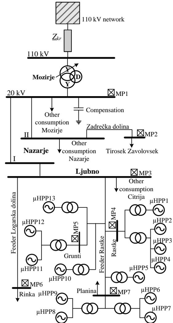
Figure 4: Simplified single-line diagram of the network.
