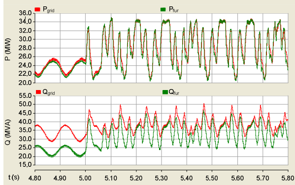
Figure 5. Waveforms of the active and reactive power of the furnace ( P_{fur} , Q_{fur} ) and active and reactive power of the network ( P_{grid} , Q_{grid} ) with “coarse regulation” before and after the start of the control algorithm; tap position 16
