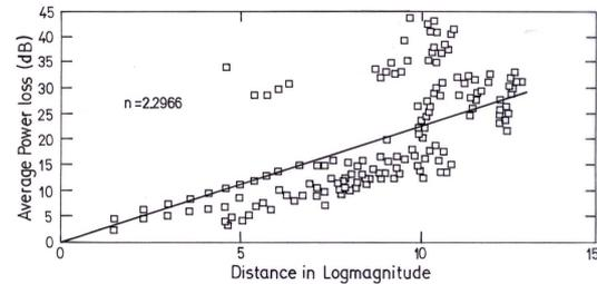
Figure 8a. Average power loss vs. Distance. [4]
