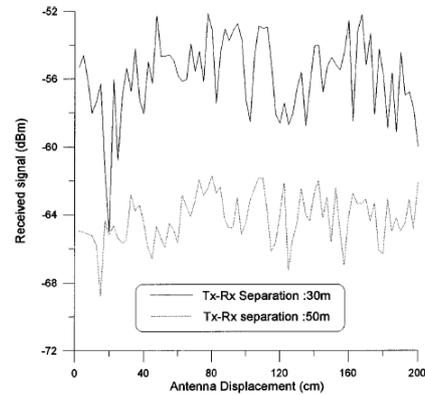
Figure 2. Received signal envelope in 2 m track antenna displacement for Tx-Rx separation 30 m and 50 m. [3]
