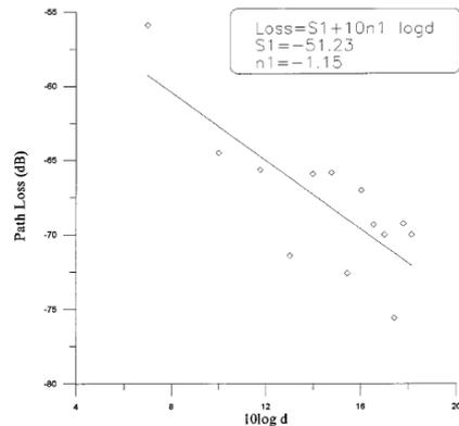
Figure 4a. Tx-Rx on the same floor without LOS conditions between them (intervening door closed). [3]
