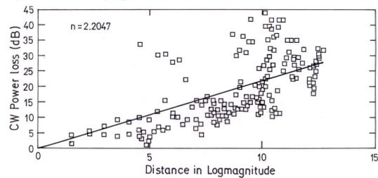
Figure 8b. CW power loss vs. Distance. [4]
