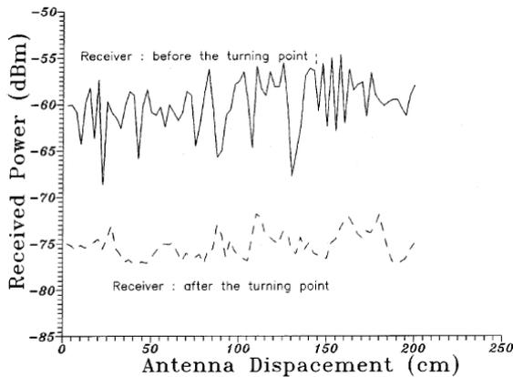
Figure 5. Comparison of envelope fading before and after the turning point in the corridor. [3]
