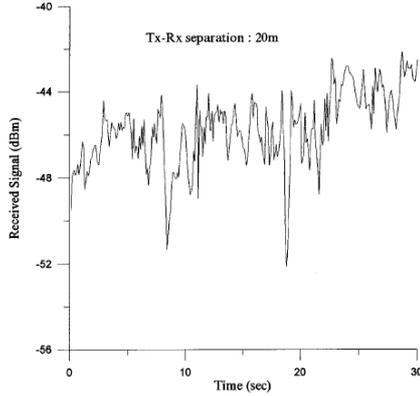
Figure 3. Received signal level due to personnel movement in a 30 second time period. [3]
