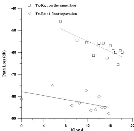
Figure 6. Comparison of measurement results for corridor and floor cases. [3]
