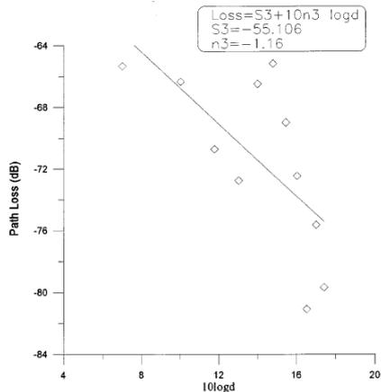
Figure 4b. Tx-Rx on the same floor – path-loss model due to temporal fading. [3]
