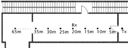
Figure 1. Configuration of the corridor
