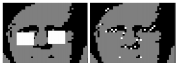
Slika 6. Območje, v katerem iščemo prisotnost svetlega območja pod kandidatoma oči (levo), in kandidati oči, ki so sprejeti na podlagi tega kriterija (desno). Figure 6. Scope for searching for the white area below eye candidates (left) and candidates that are accepted on the basis of this criterion (right).
