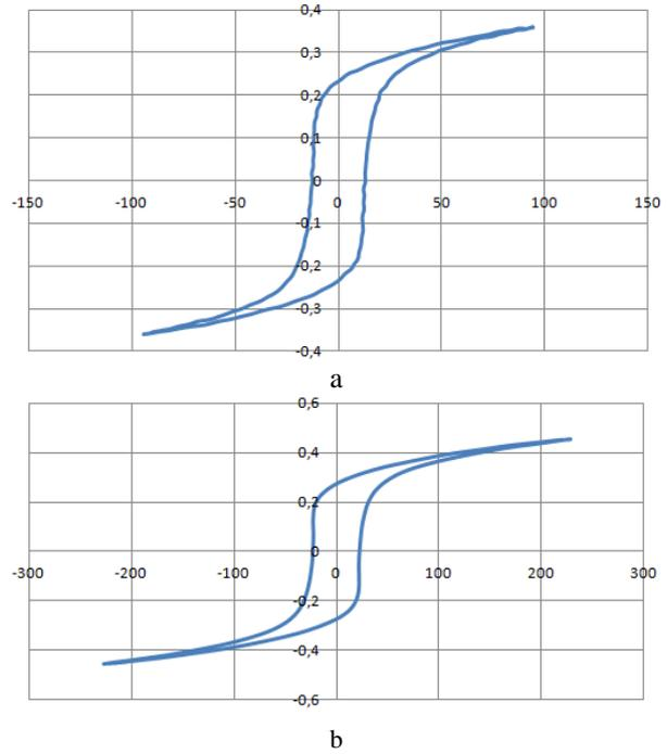
Figure 2. Experimental hysteresis loop of the 5BDSR amorphous alloy (E-type) at the 80 °C temperature:
