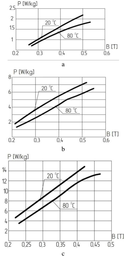
Figure 1. Loss dependence in the 5BDSR (E-type) stator core: a) on the 400 Hz magnetization reversal frequency; b) on the 1000 Hz magnetization reversal frequency; c) on the 2000 Hz magnetization reversal frequency magnetic induction and temperature.
