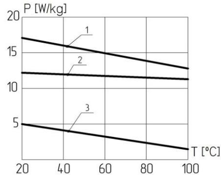
Figure 3. Temperature-dependencies of the hysteresis and eddy-current losses for the 5BDSR amorphous alloy (E-type) at a 0.45 T induction and a 2000 Hz magnetization reversal frequency:
