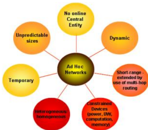
Figure 6. Wireless AD HOC Network Characteristics
