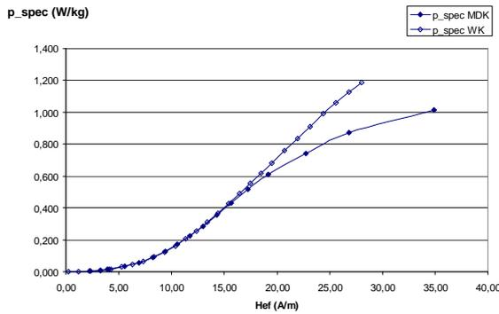
Figure 6. Specific losses (active power) vs. magnetic field strength.
