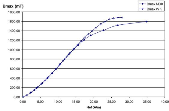
Figure 5. Magnetic flux density vs. magnetic field strength.
