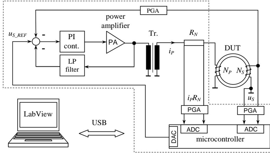
Figure 3. Block diagram of a measurement system.
