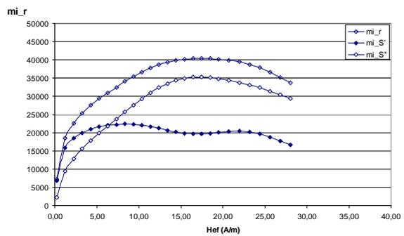
Figure 9. Complex permeability and their components  $z$  vs. magnetic field strength.
