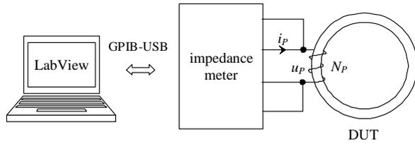
Figure 4. Measurement scheme using an impedance meter.
