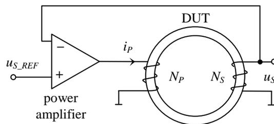
Figure 2. Measurement principle with a negative feedback voltage control loop.
