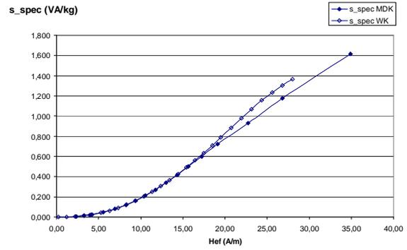
Figure 7. Specific apparent-power losses vs. magnetic field strength.
