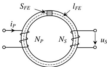
Figure 1. Toroidal core with a primary and secondary coil.
