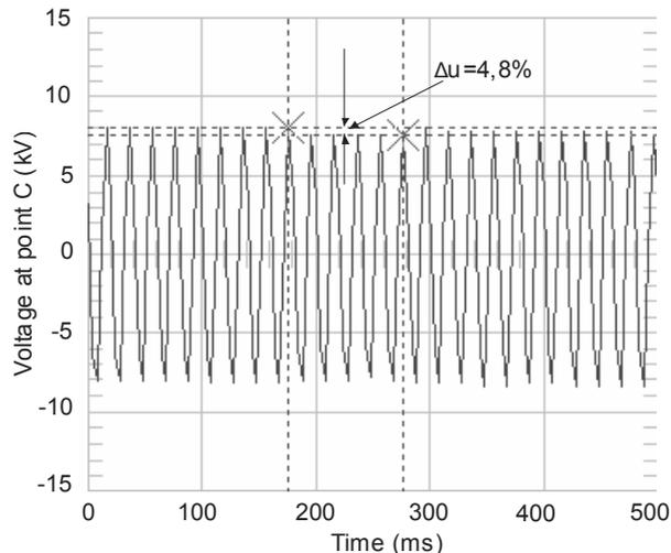
Figure 10: Voltage time at point C at short-circuit occurrence at point E
