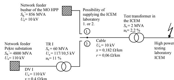
Figure 1: Possibility of supply of power laboratory
