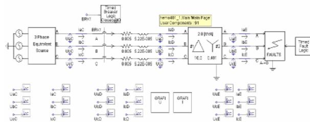
Figure 6: Simulation model in PSCAD – supply from the MO HPP
