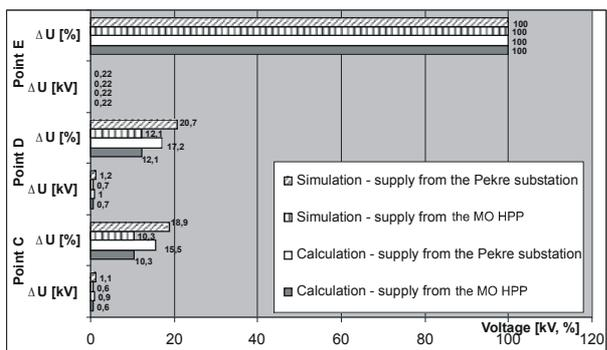
Figure 9: Comparison of voltage decreases at a three-phase short-circuit as an example of analytical calculations with PSCAD/EMTDC
