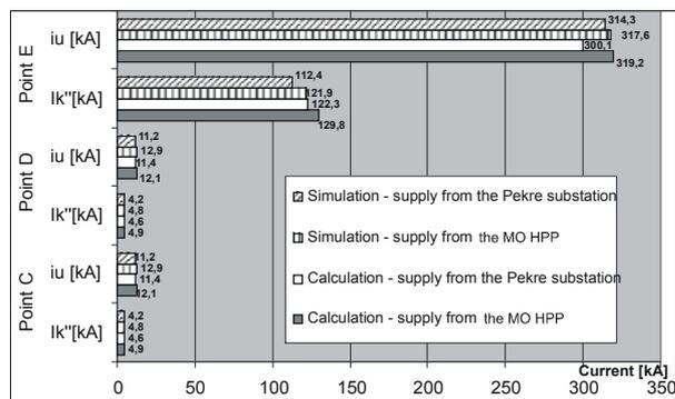
Figure 8: Comparison of the three-phase short-circuit current as an example of analytical calculations and simulations with PSCAD/EMTDC
