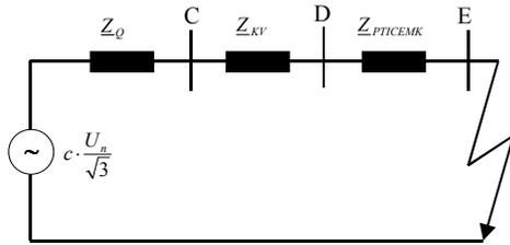
Figure 4: Equivalent network – supply from MO HPP
