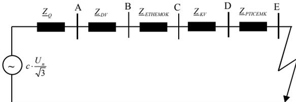
Figure 5: Equivalent network – supply from the Pekre substation
